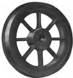
Fig. 4570. Steel Tired Wheel with Cast Steel or Wrought Iron Spoke Center. Bolted Fastening.
